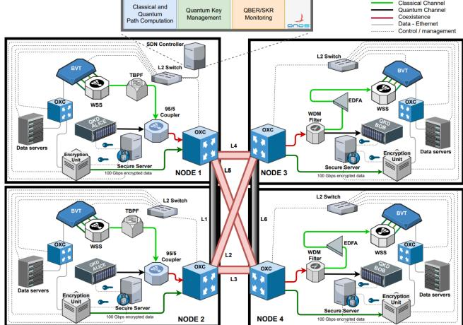
Fig.3: Trusted-node-free Dynamic QKD Network configuration two testbed. Red link: Fibre with QKD communication, Black link: Fibre without QKD communication.
