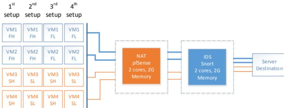
A service chain of two virtualised network functions; pfSense NAT and Snort IDS – both at 2 cores and 2G memory
