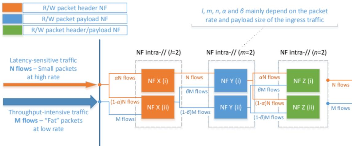
A particular case of flow-based traffic forwarding plan within a SC of three NF
