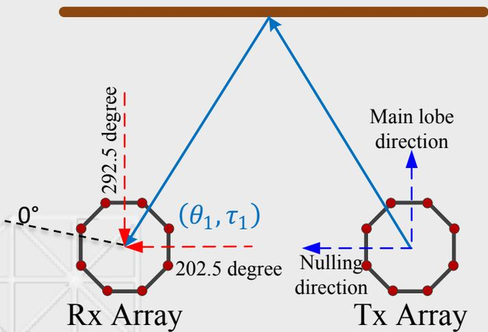
**DSI:** Tx array is  $\sim 202^\circ$  bearing from Rx array
