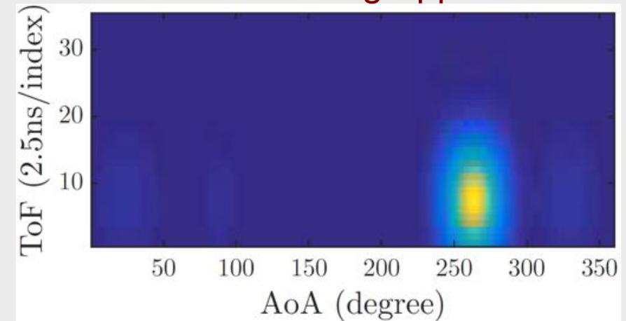
\*ToF difference between DSI and wall reflection path is 2.5 ns  $\sim$  75 cm
