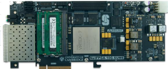
The image shows a NetFPGA-10G-SUMB board, a high-performance FPGA-based network interface card. It features a Xilinx Virtex-7 FPGA, a 10GbE SFP+ port, and various other components like memory, capacitors, and connectors. The board is labeled 'UNIVERSITY OF CAMBRIDGE NetFPGA-10G-SUMB'.
